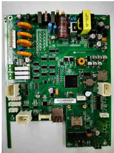
Micro SD slot of 22kW charger
