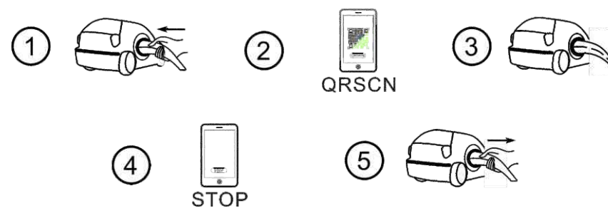
APP/RFID mode operation process flow
