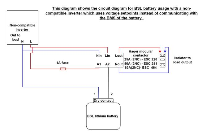
Specified contactor must be used when manually [voltage based] connecting BSL lithium batteries to non-compatible Inverter. Warranty remains for 120 months. If specified contactor is not used, warranty period is 60 months.
