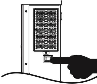
Once the unit has been properly installed and the batteries are connected well, simply press On/Off switch (located on the button of the case) to turn on the unit.
