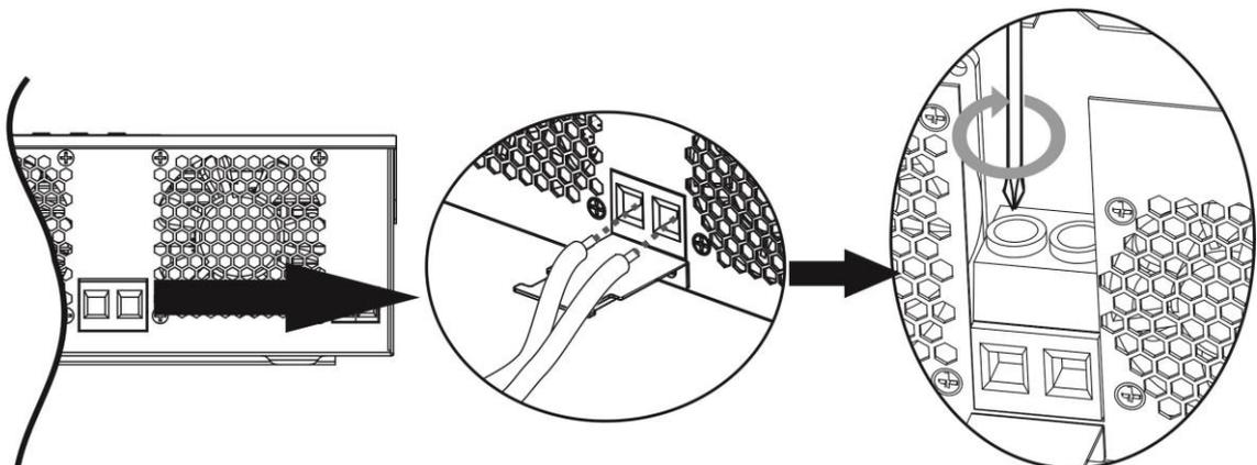
For 3KVA model, secure assembled ring terminals to the battery terminal block with the bolts properly tightened. Refer to battery cable size for torque value. Make sure polarity at both the battery and the inverter is correctly connected and ring terminals are secured to the battery terminals.
