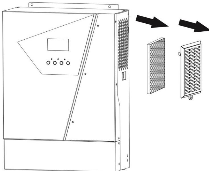
**Step 3:** Clean air filter foam and dustproof case. After clearance, re-assemble the dust-kit back to the inverter.
