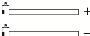
For 3KVA models, refer to recommended battery spec table to purchase separately two ring terminals and battery wires. Assemble two ring terminals with battery wires based on recommended battery cable and terminal size as grounding cable. Recommended dimensions for ring terminal is D (8.4 mm) and L (39.2 mm).
