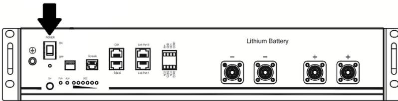
Step 3. Press more than three seconds to start Lithium battery. Output power is ready.
