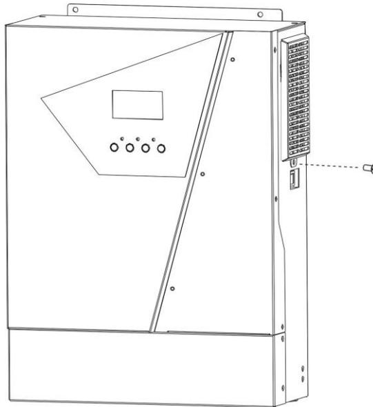
**Step 2:** Then, dustproof case can be removed and take out air filter foam as shown in below chart.
