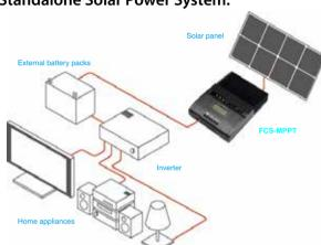
Combined MPPT technology and DSP controller, FCS-MPPT will convert best voltage to charge battery based on varied temperature. Compared to traditional solar charge controller, it allows your solar panels to operate at their optimum power output voltage, providing higher efficiency up to 98% with lower power loss.
